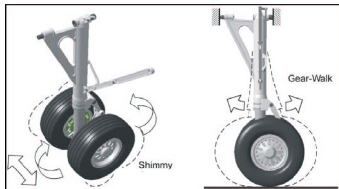
Figure 1: Shimmy and Gear Walk Phenomena [27]
